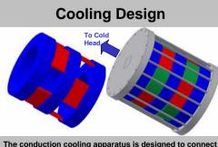
a cryocooler directly to the HTS motor. The BSCCO pancakes are wound directly to the conduction apparatus, and the bulk YBCO material plates are supported by G10.
