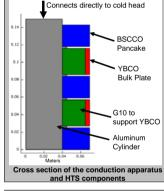
Steady state operation is designed maintain the operating temperature of the HTS materials (30 Kelvin). The cryocooler provides a refrigeration load at the cold head which connects directly to the conduction apparatus. Direct conduction cooling avoids use of liquid cryogen baths which can be problematic for mobile applications. The use of MLI wrapped around the system reduces the radiation heat load.
